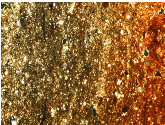
Figure 4.344: Fabric IV, DP sample 15C (PPLx10). Again note the clear colour differentiation; the sub-rounded light grey inclusions are micritic limestone.
